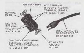
Fig. 8—Wiring of 125V Standard Plug and Receptacle
