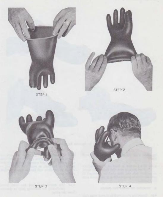
Fig. 5—Air Test Operations 1-2-3-4
