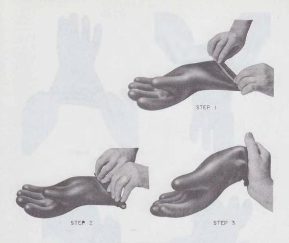
Fig. 6-Alternate Air Test
