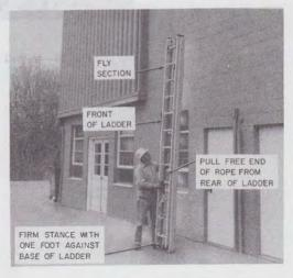
Fig. 23—Preparing to Extend Fly Section
