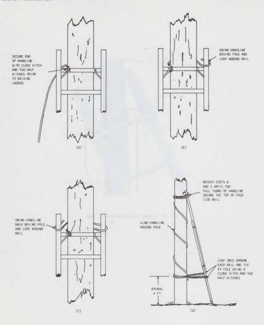
Fig. 15—Alternate Method of Lashing Ladder to Pole
