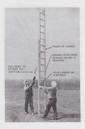
Fig. 28—Two-Person Method of Extending Fly Section
