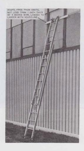
Fig. 16—Ladder Placed in Front of Window
