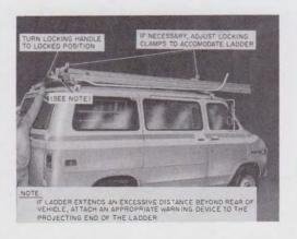
Fig. 4—Mounting Ladder on Roof-Type Ladder Bracket
