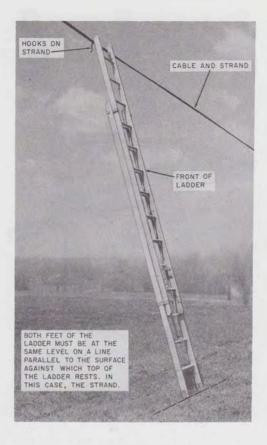
Fig. 12—Base of Ladder Properly Positioned
