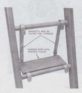
Fig. 35—B Ladder Tread in Working Position
