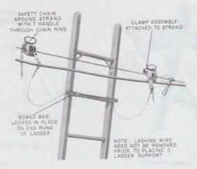
Fig. 41—D Ladder Support Attached to Strand
