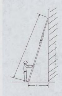
Fig. 9—Ladder Placed Against Wall
