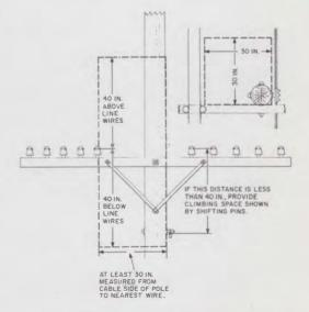
Fig. 4—Climbing Space When Drops are Attached Directly to Pole
