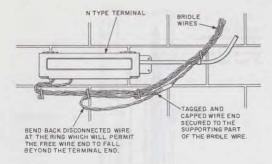
Fig. 6-N-Type Terminal Wall Mounted
