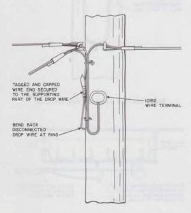
Fig. 7—101-Type Wire Terminal, Pole Mounted
