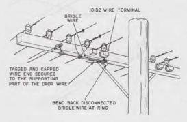
Fig. 8—Wire Terminal Mounted on Crossarm
