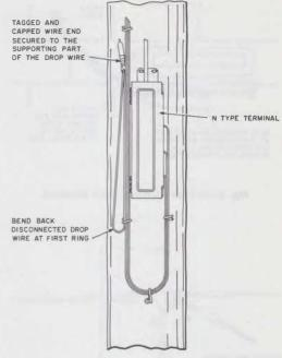
Fig. 4-N-Type Terminal, Pole Mounted
