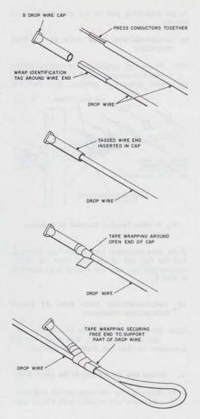
Fig. 3-Disposition of Disconnected Drop Wire
