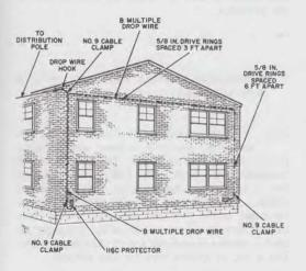
Fig. 1-Complete Wire Run on Building
