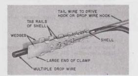
Fig. 2—D Drop Wire Clamp Assembled on Wire
