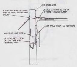
Fig. 13—Deadend Pole With Pole-Mounted Cable Terminal
