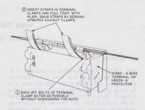
Fig. 4—Inserting Cable Supports in Terminal Clamps
