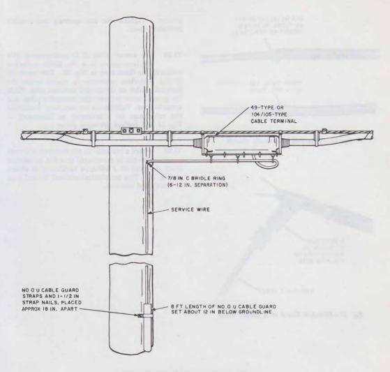
Fig. 25—Buried Plant Run Up a Pole
