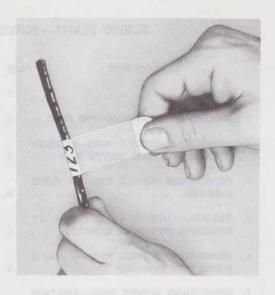
Fig. 1—♦Placing Self-Laminating Label♦
