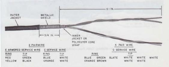
Fig. 3—Prepared Service Wire—13- or 14-Type Closure
