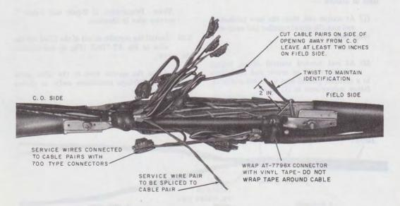
Fig. 5— Splicing Cable Pairs—13-Type Closure
