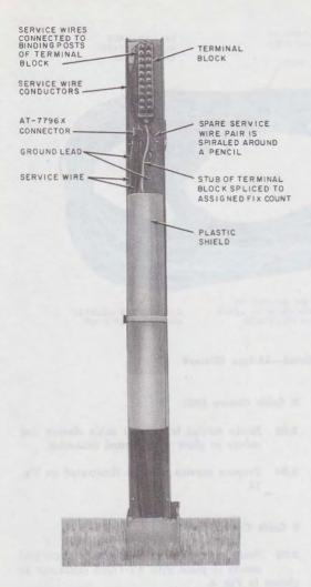
Fig. 8—\$Service Wires Terminated in RC4/72 Cable Closure\$
