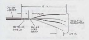
Fig. 7—Prepared Service Wire—RC4/72 Cable Closure
