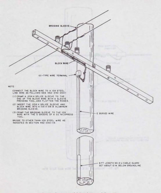
Fig. 31—Termination of E Buried Wire and Open Wire
