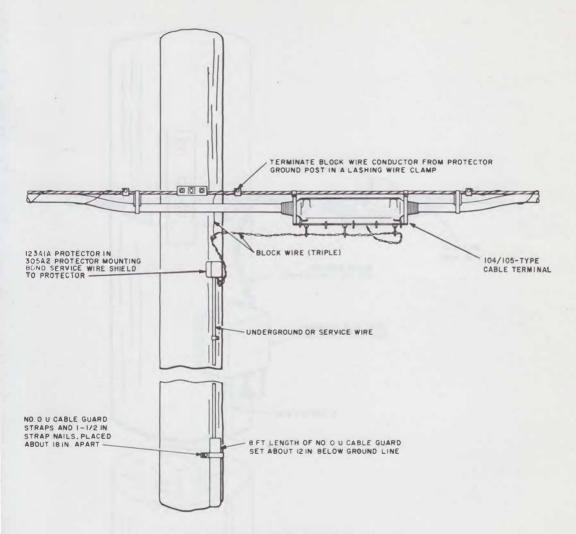
Fig. 28—Termination for Special Lightning Protection
