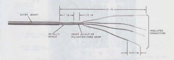
Fig. 15—Prepared Service Wire—E Cable Closure
