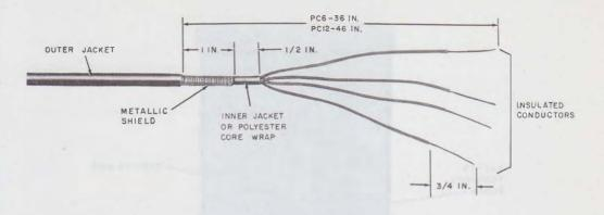
Fig. 9—Prepared Service Wire—PC6/48 or PC12/55 Cable Closure
