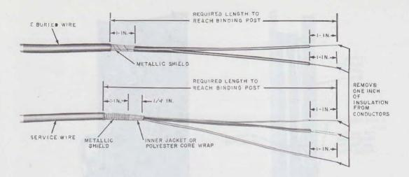
Fig. 23—▶Prepared Service Wire—D or E Buried Wire Terminal ●
