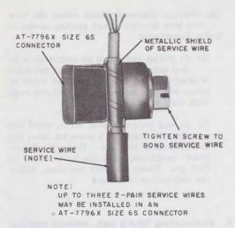
Fig. 4—PService Wire Installed in AT-7796X Connector
