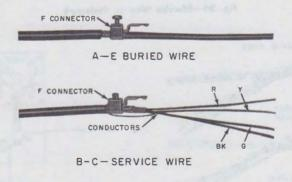
Fig. 33—₱F Connector on Service Wire¶
