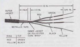
Fig. 21—Prepared Service Wire—UP200 Cable Closure
