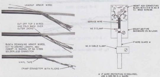
Fig. 35—Preparation of D Underground Wire (MD) for Protection or Cable Terminal Where Grounding is Required
