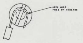
Fig. 9—Terminating Wire at Screw Terminals
