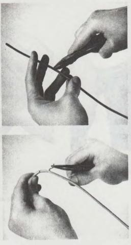
Fig. 7—Stripping D Station Wire
