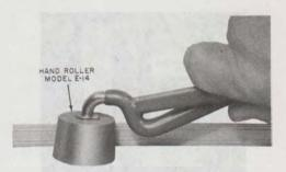
Fig. 3—Applying Roller to Wire Run
