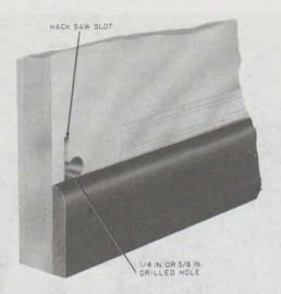
Fig. 15-Hole Through Wall for B Station Wire
