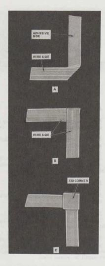
Fig. 4-90° Turn in B Station Wire
