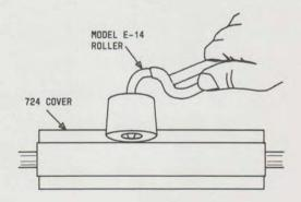
Fig. 14—Installing No. 724 Station Wire Cover
