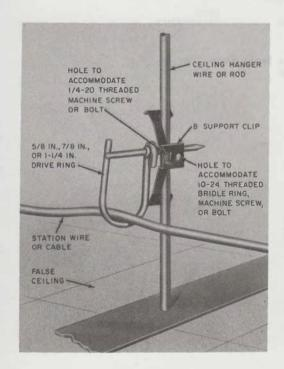
Fig. 4—B Support Clip, Installed
