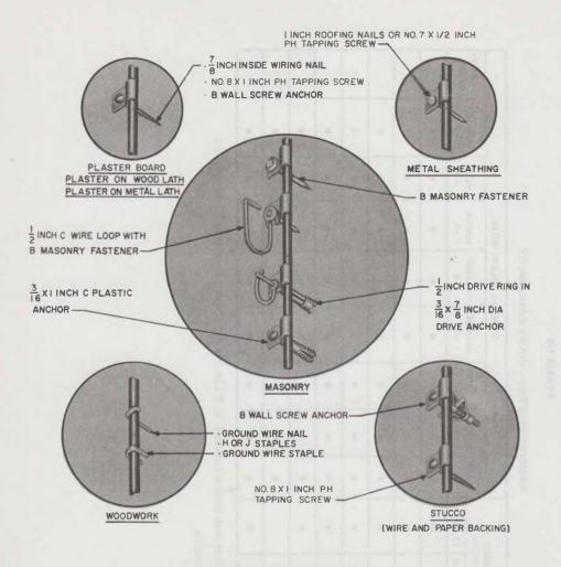
Fig. 1—Fasteners for Ground Wire
