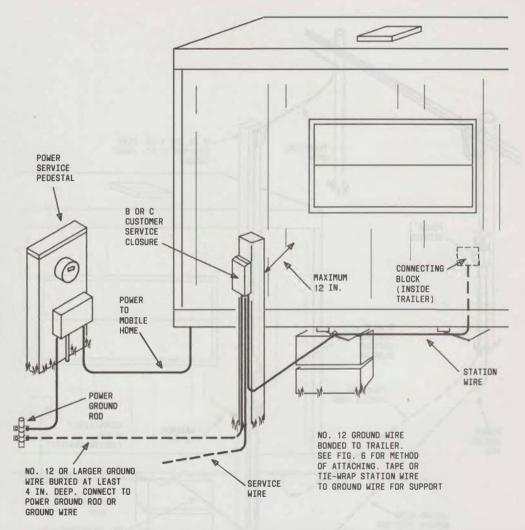
Fig. 3—Buried Service—Protector Located Witin 12 Inches of Mobile Home—Protector Grounded to Power
