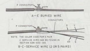
Fig. 8-F Connector on Service Wire
