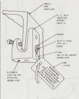
PLACE BOLT THROUGH INSULATOR SUPPORT, INSTALL BOTTOM NUT AND TIGHTEN, ATTACH INSULATOR SUPPORT TO OUTRIGGER IN USUAL MANNER, PLACE WASHERS AND TOP NUT ON BOLT, REMOVE INSULATION FROM GROUND WIRE AND BEND BARE CONDUCTOR AROUND BOLT BETWEEN WASHERS, TIGHTEN TOP NUT.
