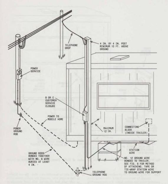
Fig. 4—Aerial Service—Protector Located Within 12 Inches of Mobile Home—Separate Bonded Power and Telephone Grounds
