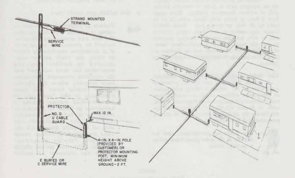
Fig. 1—Typical Buried Service Distribution
