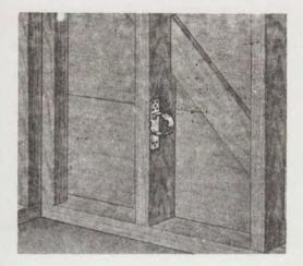
Fig. 14—Stud-Mounted 63A Bracket
