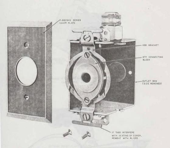
Fig. 11-47-Type Connecting Block Mounted in Standard Electrical Outlet Box (Front View)
