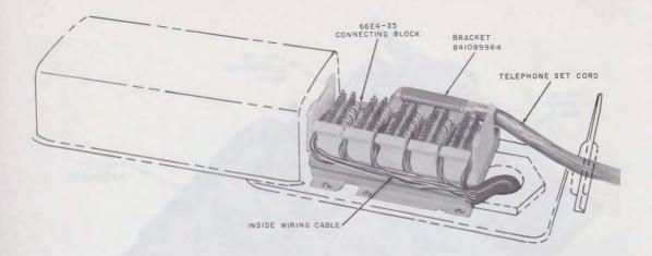
Fig. 4-66E4-25 Connecting Block Installed in Commercial Fitting
