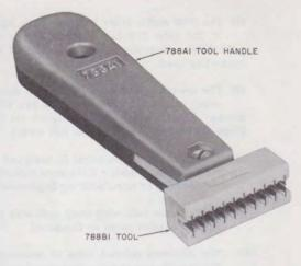
Fig. 8—5-Pair Insertion Tool
