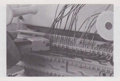
Fig. 17—Cutting Excess Wire
