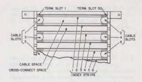
Fig. 12—Numbering Plan for 88-Type Wiring Block
