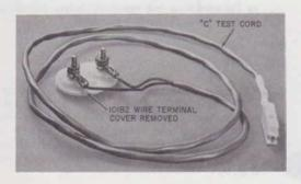
Fig. 7—C Test Cord and Terminal Block
