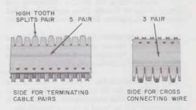
Fig. 3—88-Type Connecting Block
