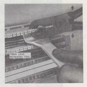
Fig. 26-\$788K1 Lead Retention Tool\$
