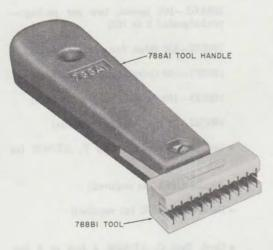
Fig. 9—5-Pair Insertion Tool
