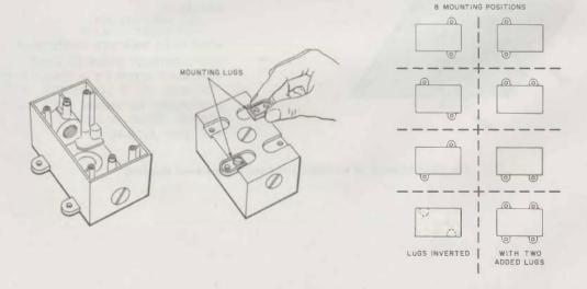
Fig. 22—KS-19316, List 6, Housing Box Showing Reversible Mounting Lugs
