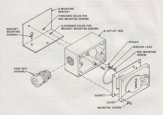
Fig. 56—Assembly of B Weatherproof Male Jack to B Outlet Box and B Mounting Bracket
