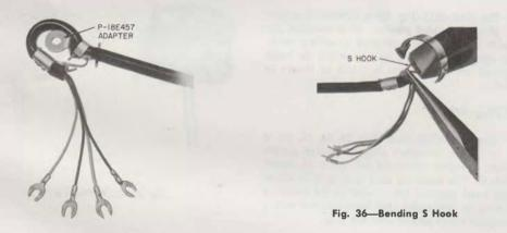
Fig. 35—Early Model D4BP Cord and Adapter
