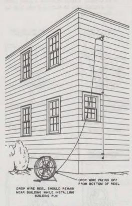
Fig. 3—Drop Wire Attached to Building
