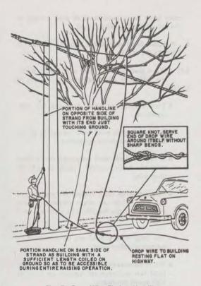
Fig. 7—Drop Wire Tied to Handline
