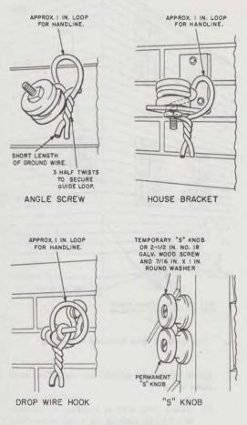
Fig. 2—Temporary Guide Loop
