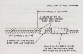
Fig. 8—Alternate Tie to Prevent Snagging
