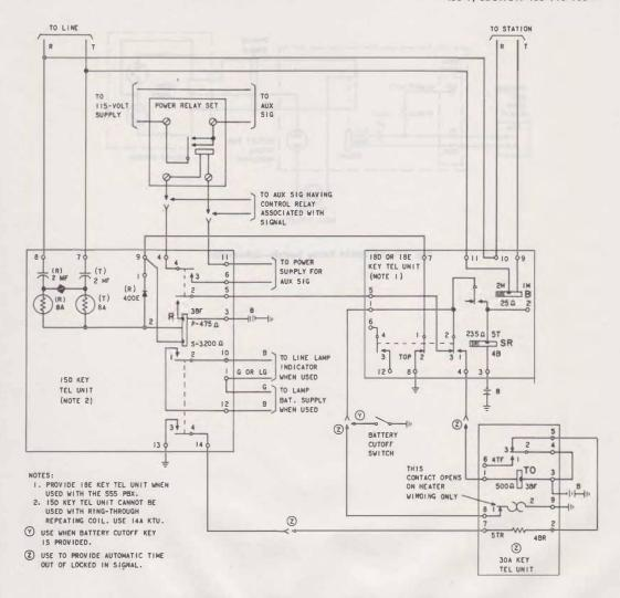
Fig. 26—Connections and Circuit Operation for Continuous Auxiliary Signals
