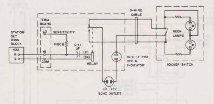
Fig. 27—KS-20614 Relay Switch—Schematic
