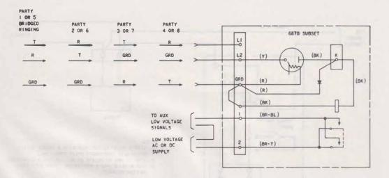
Fig. 25—Noncontinuous Low Voltage Auxiliary Signal
