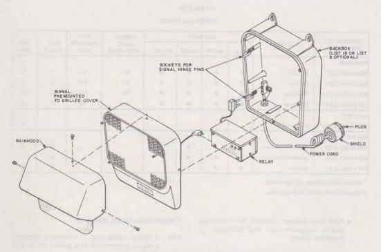
Fig. 1—Exploded View of Assembled Signal Using Relay
