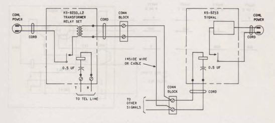
Fig. 22—KS-8233, List 2 Transformer Relay Set
