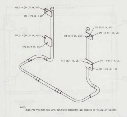
Fig. 11-77C Apparatus Mounting
