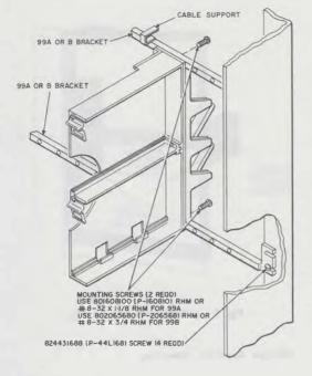
Fig. 6—69-Type Apparatus Mounting on a 99-Type Bracket
