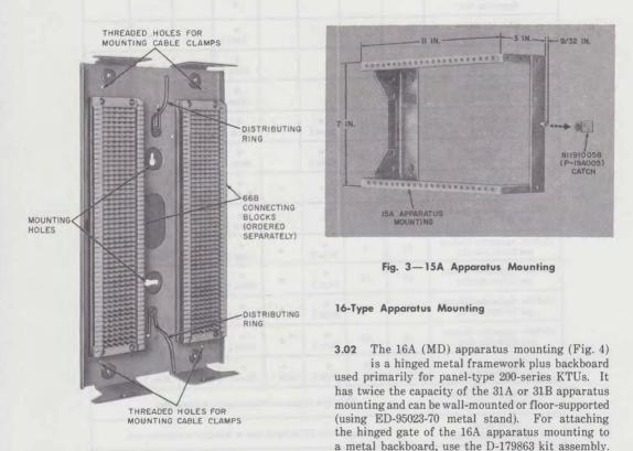
Fig. 2—Typical 115-Type Apparatus Box with Distributing Rings and Connecting Blocks Installed
