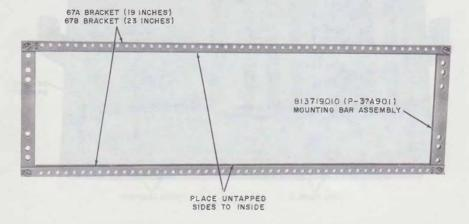
Fig. 44—67-Type Brackets for Mounting Panel Type 200-Series Key Telephone Units
