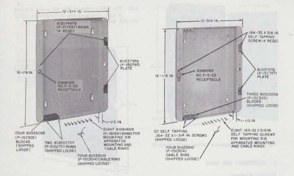
Fig. 20—177A Aluminum Backboard Assembly (MD)
