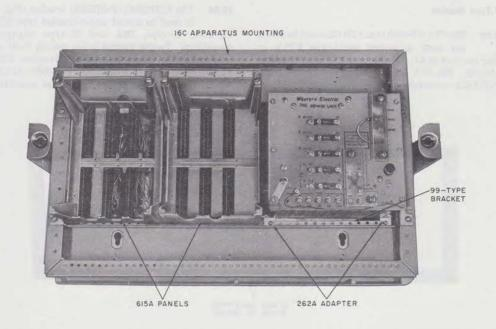
Fig. 42—16C Apparatus Mounting with 615A Panels Mounted on 99-Type Brackets and 20-Type Power Unit Mounted on 262A Adapter
