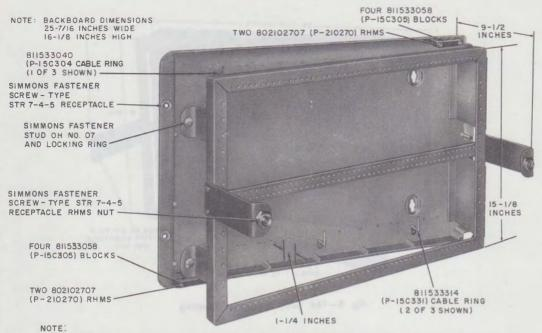
MOUNTING MAY BE INVERTED 180 DEGREES WHEN REQUIRED TO OPEN GATE TO THE LEFT.
