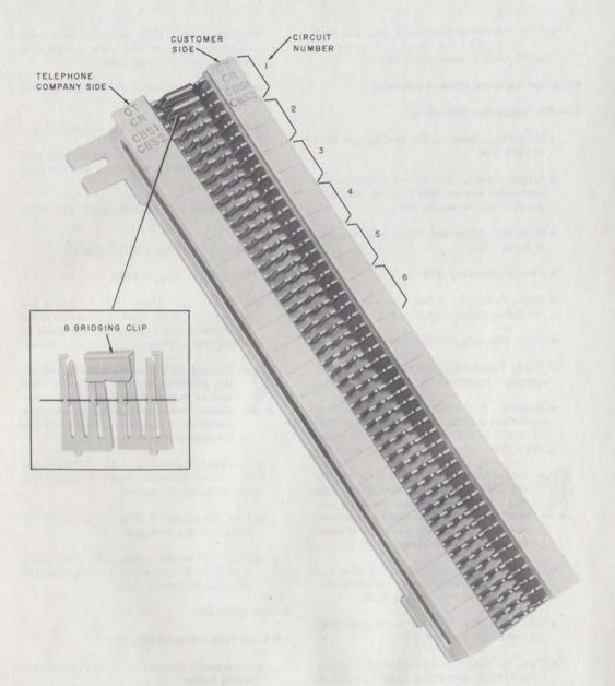
Fig. 3—Typical Interface Connecting Block
