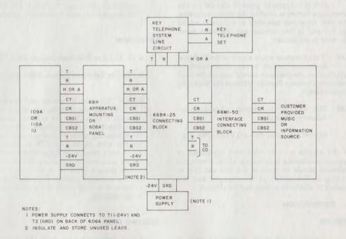
Fig. 1—Block Diagram—Voice Connecting Arrangement LVH
