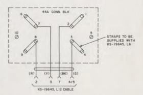
Fig. 29-KS-19645, List 6 Recorder Connector
