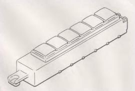
▶Fig. 7—111A—White plastic blank intended for use in the No. 3640A and 3641A type telephone sets to fill the space reserved for additional No. 635\*2 (rectangular buttoned) keys. The width of the blank is the same as that of one of the keys.
