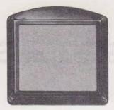
▶Fig. 8—50K—Metal mounting plate, 4-11/16 inches high by 4-3/4 inches wide. Equipped with a card frame, card holder assembly, Allen head mounting screws, and plastic window protector for the instruction card. Early production models will be provided with slot head mounting screws, and without the plastic window. The chrome plated 50K apparatus blank replaces the 50L apparatus blank. For all type coin collectors.
