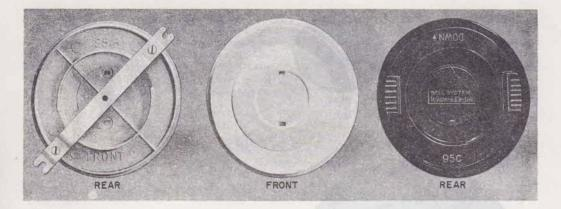
Fig. 5-95B and 95C (Early Model)-95C replaces 95B. 95C (early model) equipped with ribs which provides frictional fit to dial mounting bracket. It will fit only sets having 2 point suspension. 95B provided with mounting bracket and screws. All apparatus blanks are provided with number card holder group. For 500-type telephone sets.
