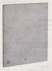
Fig. 14—107B—Clear anodized aluminum sheet with drawn edges, 12-1/2 inches high by 9-1/2 inches wide. For covering opening of 113-type apparatus box in absence of 750-type telephone set and 114-type apparatus box in absence of 752-type telephone sets. Provided with mounting brackets and screws.
