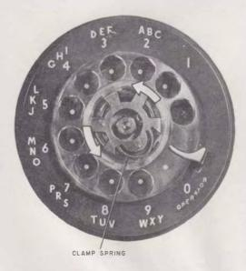
Fig. 5 — Replacing Plastic Fingerwheel
