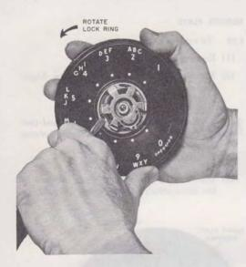
Fig. 7 — Lock Ring Removal
