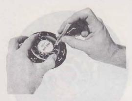
Fig. 4 — Removing Plastic Fingerwheel
