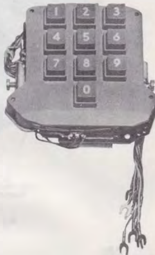
Fig. 1—10-Button 25-Type Nonconvertible Dial, Front View
