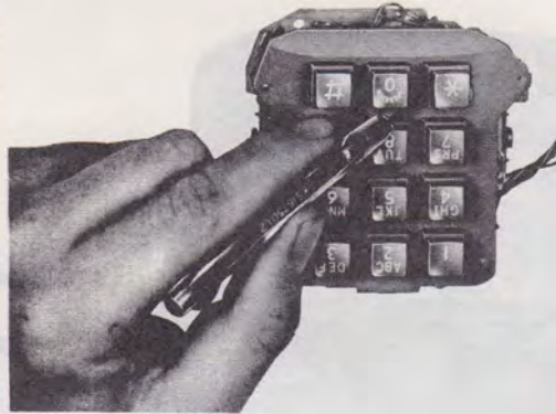
Fig. 8—Removing Special Service Button
