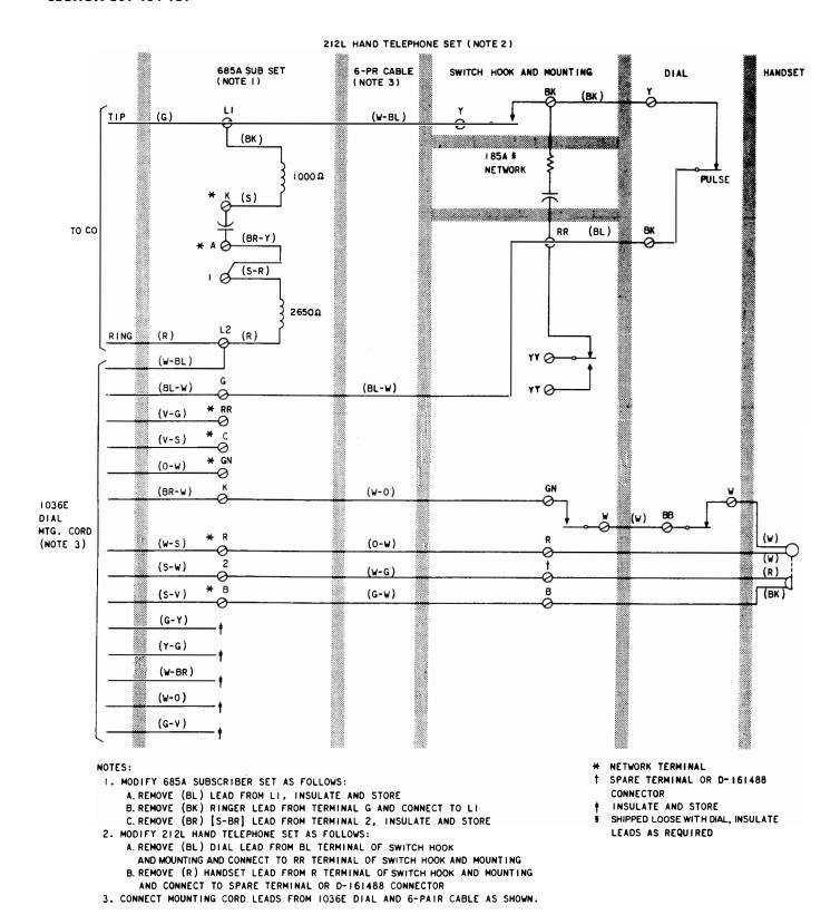
Fig. 5—1036E Dial, Connections to 212L Hand Telephone Set
