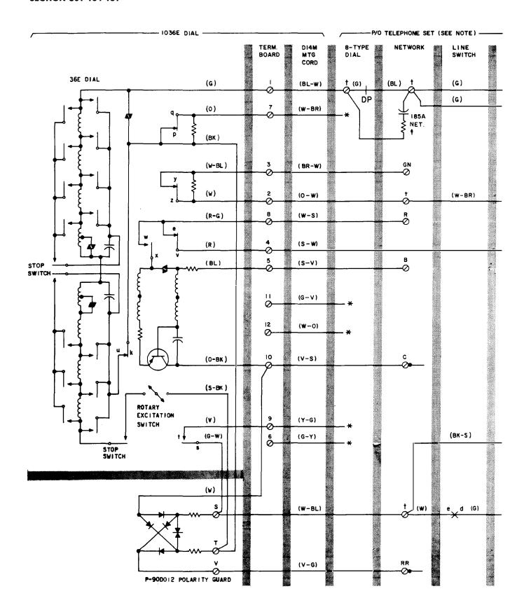
Fig. 8—♦1036E Dial, Connections to 636CA or 637DA Telephone Set (Sheet 1 of 2)♦
