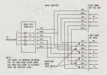
Fig. 4—Layout of 304A Adapter
