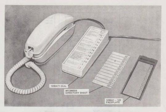
Fig. 6—1200AT1 Dial With Faceplate and Directory Sheet Removed
