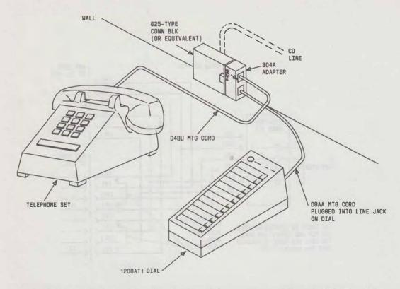
Fig. 5—Optional Installation for Single Line Modular Desk Type Telephone Set With D-180882 Kit of Parts
