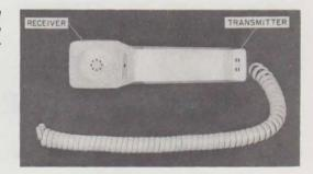
Fig. 1—M1A Handset With H4DU Handset Cord Connected
