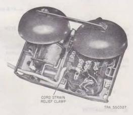
Fig. 7—Top View, Mounting Cord Entering from Left
