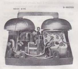
Fig. 5—Top View, Inside Wire Entering through Rear
