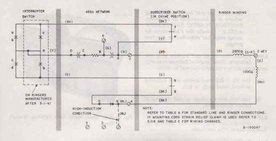
Fig. 4—FIA Ringer, Schematic
