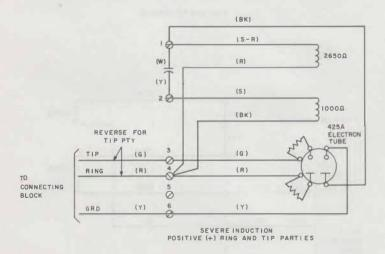
Fig. 3—L1A (MD) and L1AM Ringer, Connections (Sheet 2 of 3)
