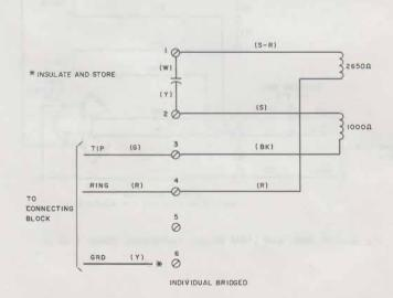
Fig. 3—L1A (MD) and L1AM Ringer, Connections (Sheet 1 of 3)
