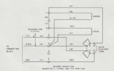
Fig. 3—L1A (MD) and L1AM Ringer, Connections (Sheet 3 of 3)
