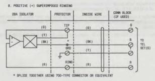
Fig. 4—₱28A Isolator Connections for Tip Party (4-Conductor Wiring) ●
