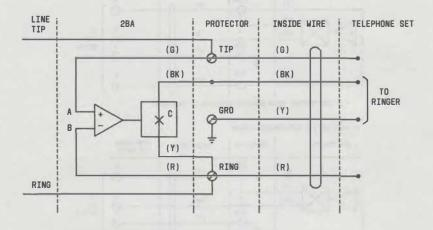
ISOLATOR TRIGGERS ON VOLTAGE DIFFERENTIAL BETWEEN A AND B AND SWITCHES RINGING CURRENT THROUGH AT C TO TELEPHONE SET. THROUGH RINGER, AND BACK TO GROUND
