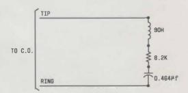
Fig. 2-1A Termination Unit, Connections
