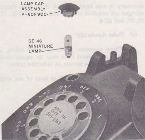
Fig. 9—Lamp Assembly, 500H/P Telephone Set
