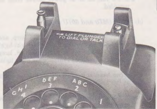
Fig. 5—500F or 501F Telephone Set, Plunger Switch
