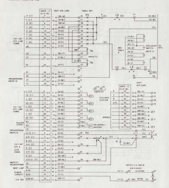
Fig. 2-\$2565LKMS Telephone Set, Connections (Sheet 1 of 2))
