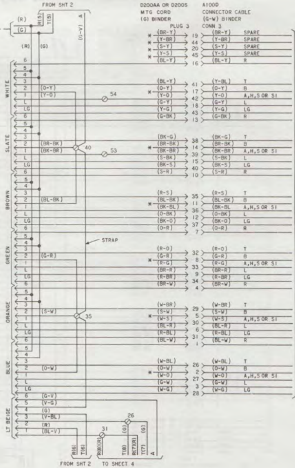
Fig. 3—Module and Connector Cable Arrangements (Sheet 3 of 5)
