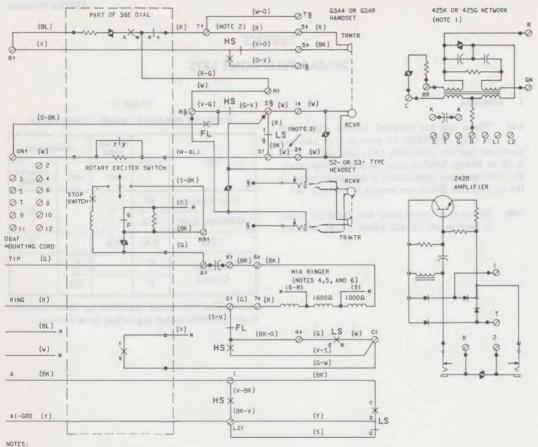
1. 425G NETWORK ELECTRICALLY THE SAME AS 425K NETWORK, THE 425K NETWORK PROVIDES S AND T TIE POINT TERMINALS.
