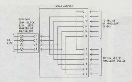
Fig. 32—Schematic of 267A Adapter
