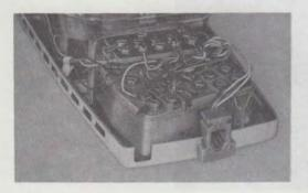
Fig. 50—2554B2M Telephone Set Base With Handset Cord Jack Installed
