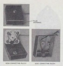
Fig. 8—625A and 625C Modular Connecting Blocks
