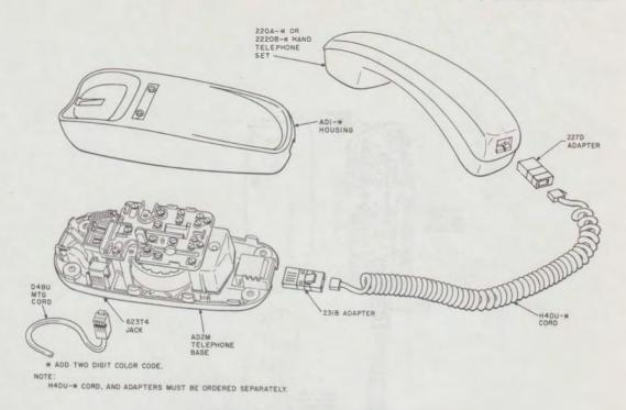
Fig. 4—AD2 Telephone Base With 220A or 2220B Hand Telephone Set
