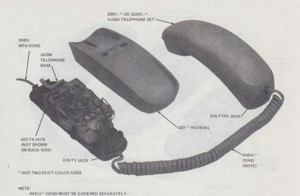
Fig. 6—AD3 Telephone Base With 220C, 226A, 2220C, or 2226A Hand Telephone Set
