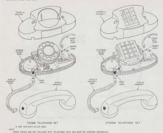
Fig. 3-702BM and 2702BM Telephone Sets
