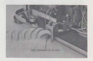
Fig. 37—123A Apparatus Blank Installed on 2500D1M Telephone Set Base
