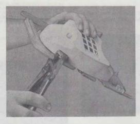
Fig. 53—Notching 2702B1 Housing and Using Check Gauge
