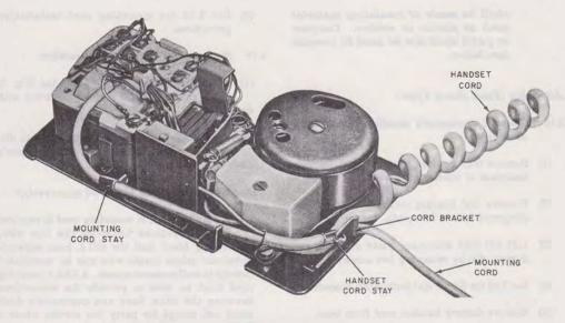
Fig. 5—Installation of Mounting and Handset Cords
