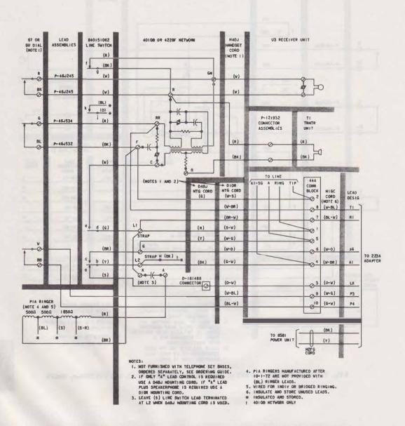
Fig. 10—Wiring for 1A1, 1A2 KTS or 4-Type Speakerphone and 1A1, 1A2 KTS (Rotary Dial) 4
