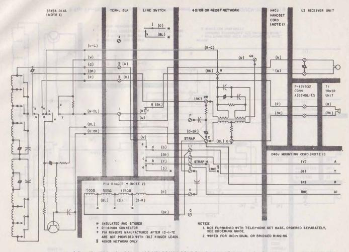
Fig. 12—Wiring for 1A1 or 1A2 KTS TOUCH-TONE Dial Equipped Telephone Set Base (
