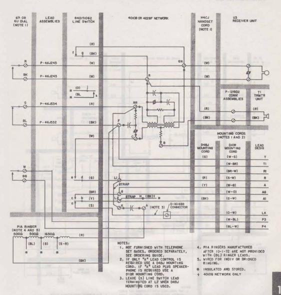
♦ Fig. 9—Wiring For 1A1, 1A2 KTS or 3-Type Speakerphone and 1A1, !A2 KTS (Rotary Diai) ♦
