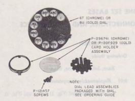
Fig. 2—6T or 6U Dial and Associated Parts
