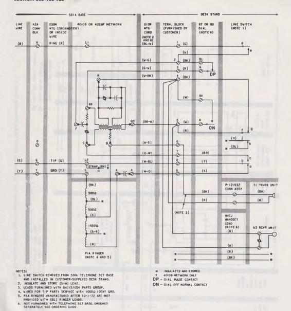
Fig. 14—Desk Stand Type Telephone Set Connections (With D10R Mounting Cord)
