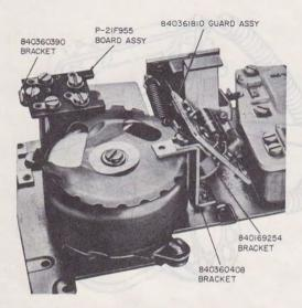
♦ Fig. 4—Installation Location of Components to Add TOUCH-TONE® Dial and Polarity Guard Features €
