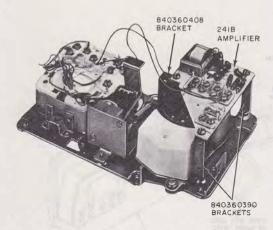
Fig. 7—Installation of D-180409 Kit of Parts
