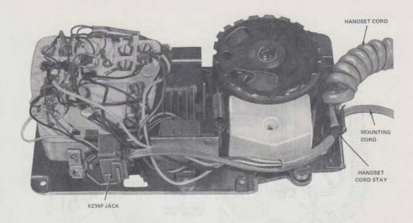
Fig. 5—Installation of Mounting Cord Using D-180778 Kit of Parts
