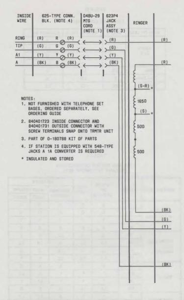
Fig. 10—581A Telephone Set Base, Wiring for 1A1, 1A2 KTS Using D-180778 Kit of Parts (Rotary Dial, Current Version) (Sheet 1 of 2)
