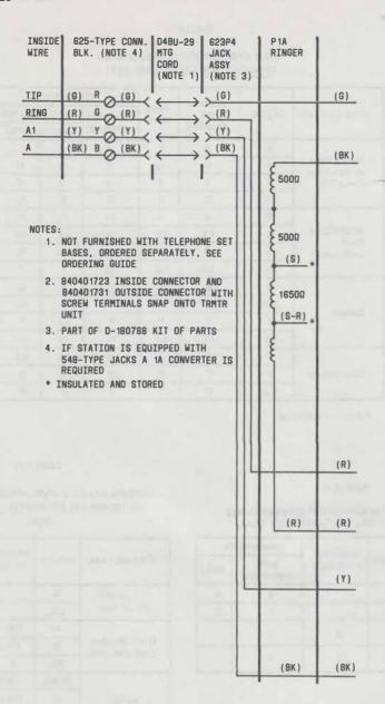
Fig. 15—Wiring for 1A1, 1A2 KTS Using D-180788 Kit of Parts (TOUCH-TONE Dial, Current Version) (Sheet 1 of 2)
