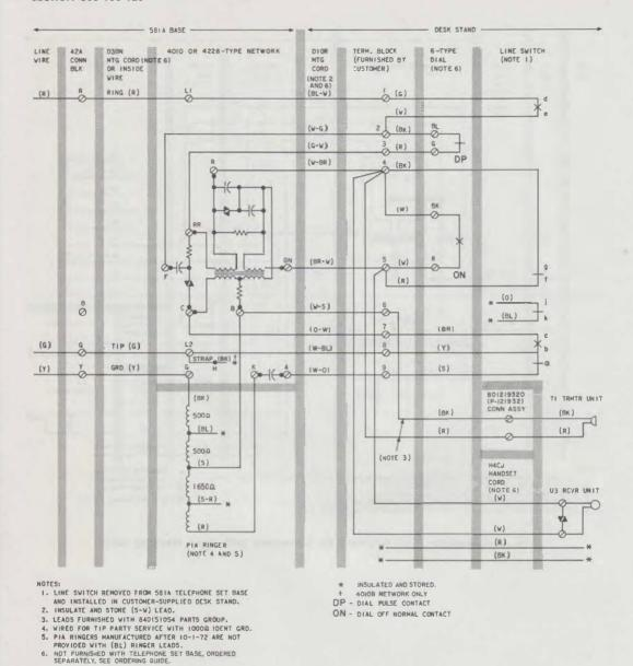
Fig. 18—Candlestick Type Telephone Set Connections Wired for Tip Party Identification (With D10R Mounting Cord)
