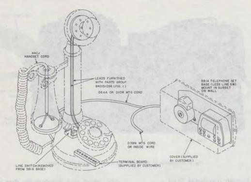
Fig. 6—Typical Installation of Candlestick Type Telephone Set
