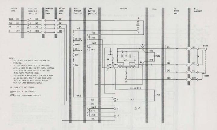
Fig. 9-10A Telephone Set Wired for 1A1 or 1A2 KTS
