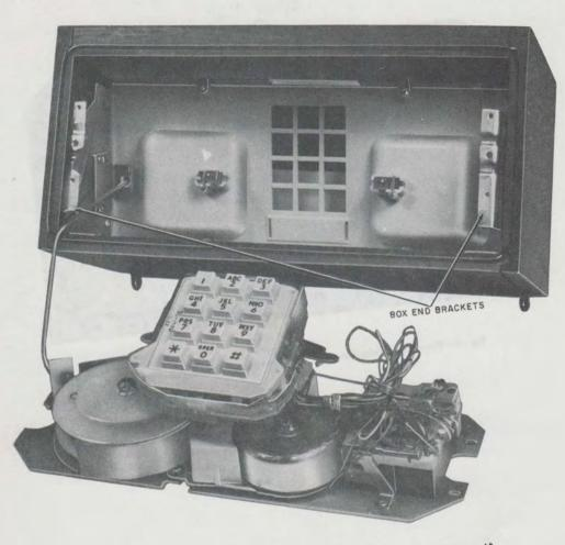
Fig. 6—2910A Telephone Set with Telephone Set Base Removed♥
