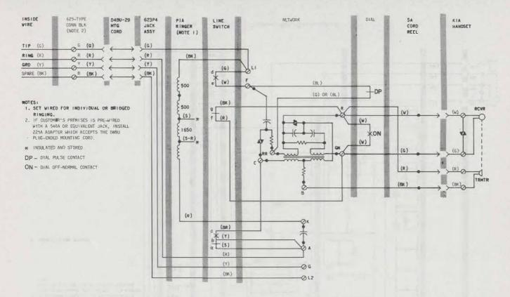
Fig. 7—₱910A Telephone Set, Connections♥
