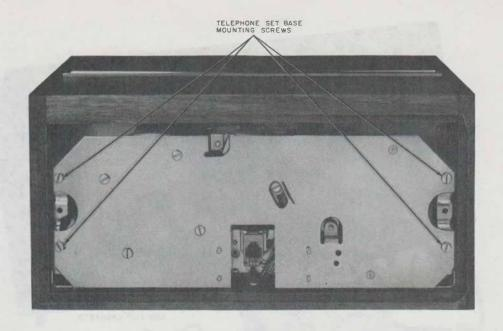
Fig. 5—Removing Telephone Set Base (910A or 2910A Telephone Set)
