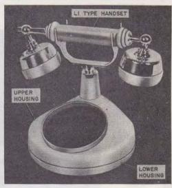
Fig. 2—Customer-Owned Components 940A or 940B
