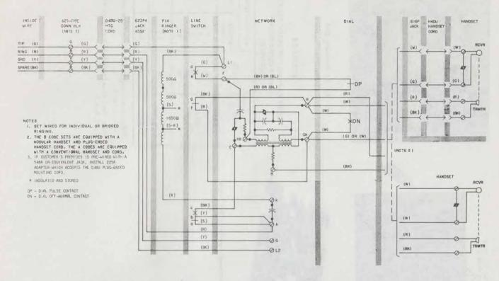
Fig. 7-♦881A102, 881B102, 881A103, 881B103, 881A104, or 881B104 Telephone Set, Connections€
