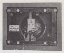
Fig. 6—Removing Dial
