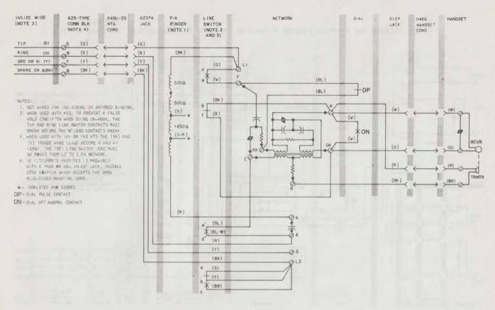
Fig. 9-\$881C102, 881C103, or 881C104 Telephone Set, Connections
