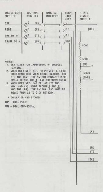
Fig. 9-\$881C105, 881C107, or 881C108 Telephone Set, Connections (Sheet 1 of 2)
