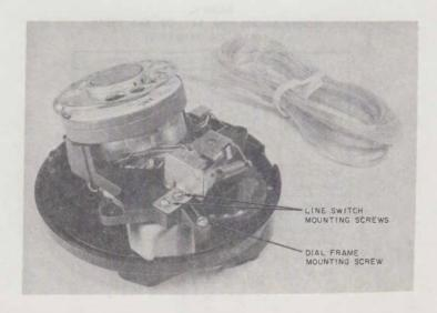
Fig. 3—Removing Line Switch and Dial Mounting Frame
