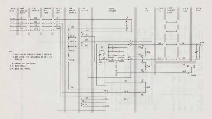
Fig. 8—♥881B105 (MD), 881B106 (MD), 881B107 (MD), or 881B108 (MD) Telephone Set Wired for 1A1 or 1A2 KTS♥
