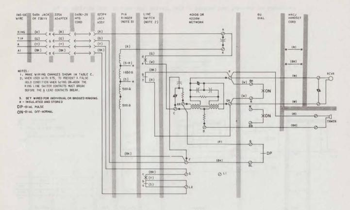
Fig. 6—♥881A105 (MD), 881A106 (MD), 881A107 (MD), or 881A108 (MD) Telephone Set Wired for 1A1 or 1A2 KTS♥
