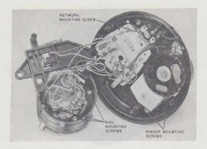
Fig. 4-Removing Dial, Network, and Ringer
