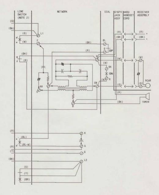
Fig. 9-\$81C105, 881C107, or 881C108 Telephone Set, Connections (Sheet 2 of 2)
