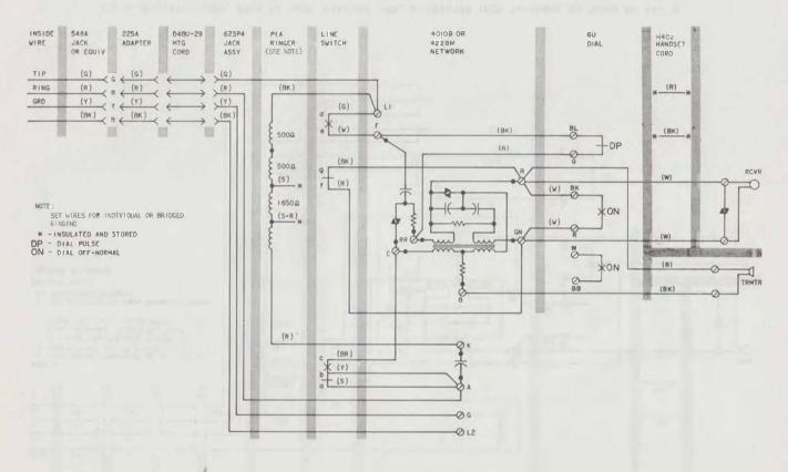
Fig. 5—₱881A105 (MD), 881A106 (MD), 881A107 (MD), or 881A108 (MD) Telephone Set, Connections
