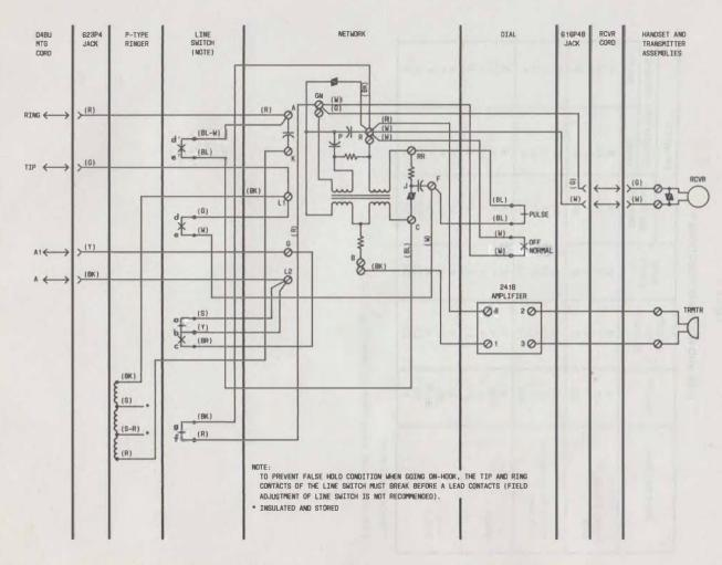
Fig. 5-952A1-03 Telephone Set, Connections For 1A1 or 1A2 KTS
