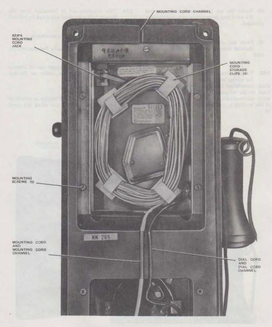
Fig. 2-952A1-03 Telephone Set, Rear View
