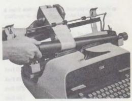
Fig. 9—Placing 1B Cartridge in Typewriter
