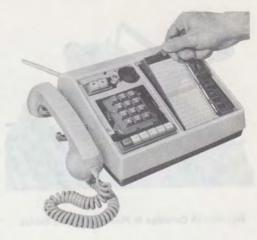
Fig. 8-Removal of 1B Cartridge
