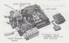
Fig. 6—#2671B1M Telephone Set, 635-Type Key and 35S3A Dial Removed#
