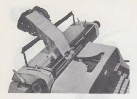
Fig. 10—1B Cartridge in Place For Typing Entries
