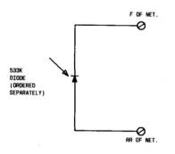
Fig. 5—Installing Diode for Dial Restriction
