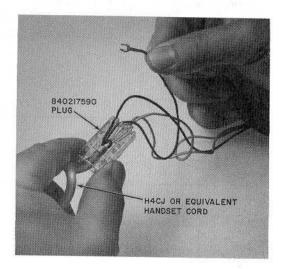
Fig. 4—Installation of Spade-Tipped Handset Cord Leads
