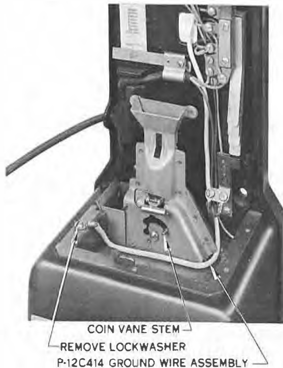
Fig. 7 — Method of Grounding Housing Assembly, Indoor Booth
