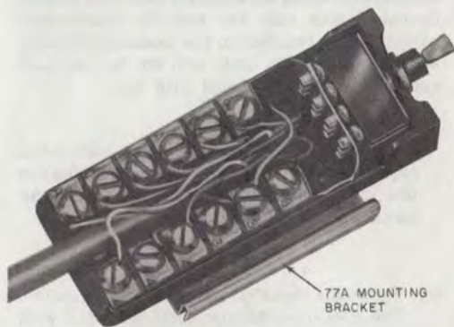
Fig. 6—Interior View of KS-21254, List 4 Key (MD) Showing Leads Terminated
