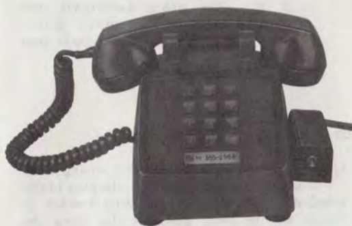
Fig. 5—KS-21254 Type Key (MD) Installed With 2500-Type Telephone Set
