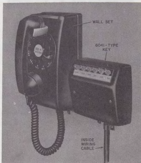
Fig. 4—Typical Installation of 6041-Type Key
