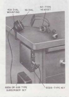
Fig. 1—Typical 4A Key Equipment Installation
