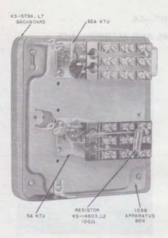
Fig. 2—Battery Feed Filter and Holding Relay
